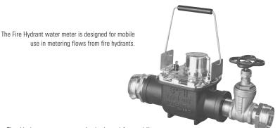
The Fire Hydrant water meter is designed for mobile use in metering flows from fire hydrants. The meter measures a wide flow range to maximize revenue. It meets or exceeds the latest performance requirements of AWWA. Maximum flow rates may be exceeded by 25% for intermittent flows.
